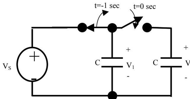
The capacitor on the right is initially discharged ( $V_2=0$ ), and the one on the left is charged to a voltage  $V_s$ . The switch on the left is opened at  $t=-1$  sec, and the switch on the right closes at  $t=0$  sec.
